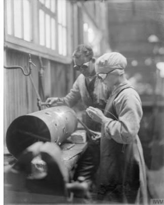
Fig. 12. A member of Queen Mary's Army Auxiliary Corps (QMAAC) acetylene welding at a Royal Air Force engine repair shop at Pont de l'Arche, France, in 1919; Olive Edis; “Q8117”; *The Imperial War Museum*; [iwm.org.uk](http://iwm.org.uk); 1919; Web; 14 Jan. 2016.
